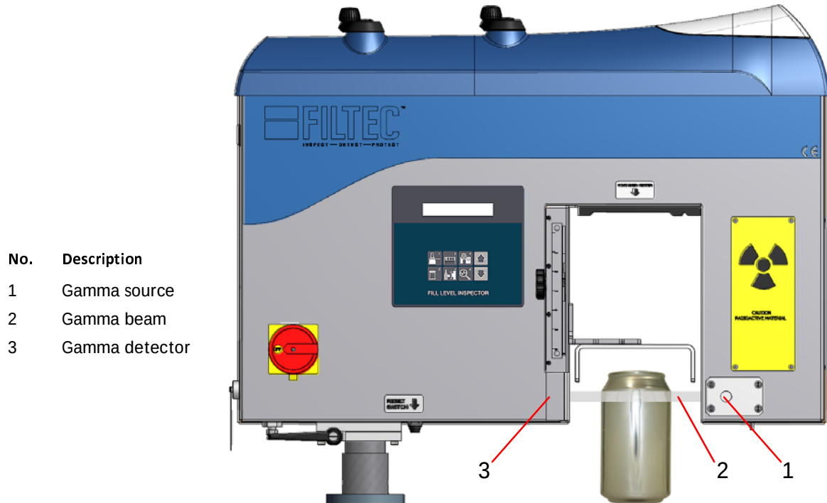
Figure 2-2. Scanning the Container
